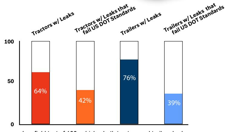
In a field test of 100 vehicles both tractors and trailers had leaks that would fail DOT standards
